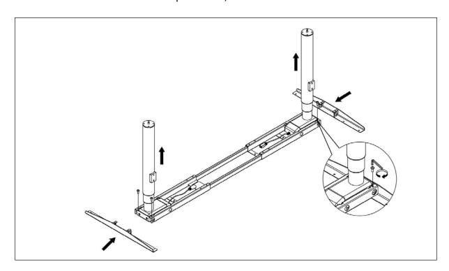
**Step 4** Install the leveling pads
