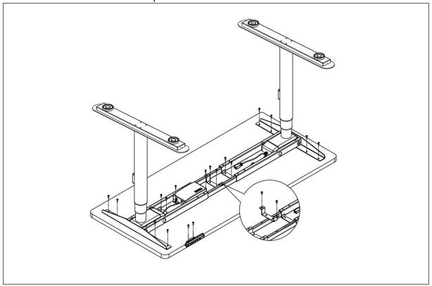
**Step 6**Mount the control box to the frame; Fix the handset with 2 pcs screws ST4x20 Zipped the cables with cable tie.
