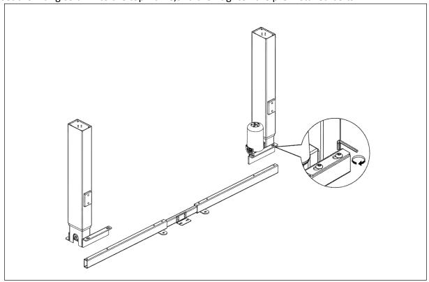
**Step 3**Install the two table feet with Screws 8 pcs M6x16, Install the 4 pcs leveling pads
