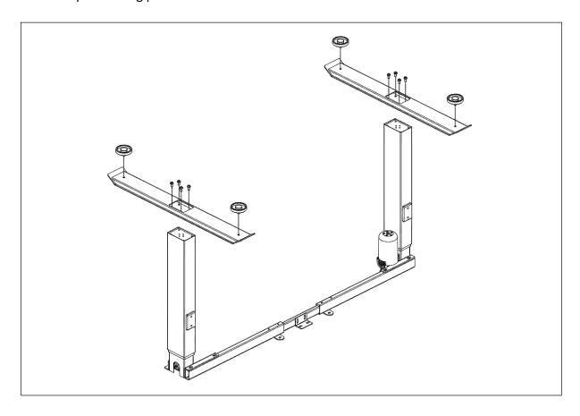
**Step 4**Install the two side brackets with Screws 4 pcs M6x12,
