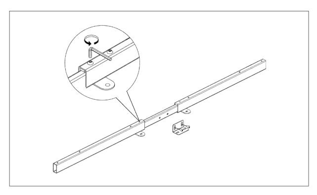
**Step 2**Inset the lifting column to the top frame,and then tighten the pre-installed bolts
