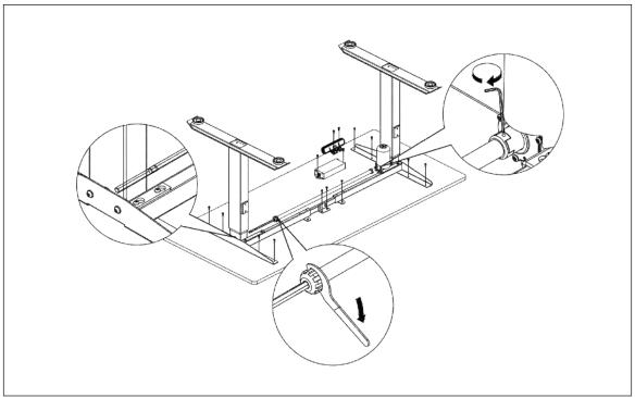
**Step 6**Connect all power supplies,then tighten the bolts on the frame Zipped the cables with cable tie.
