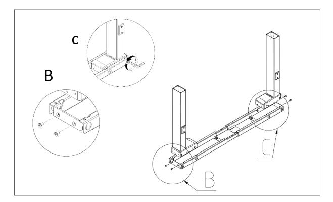
**Step 3**Install the two table feet with Screws 8 pcs M6x16, Install the 4 pcs leveling pads
