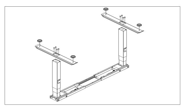
**Step 4**Install the two side brackets with Screws 4 pcs M6x12,
