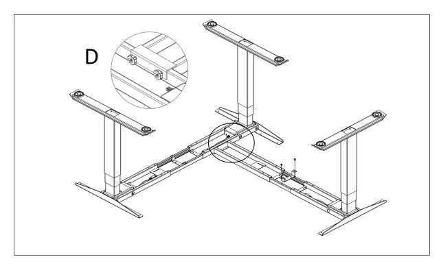
**Step 6**Mount the tabletop and fix it with 19 pcs screws ST4x20
