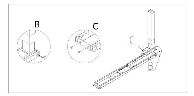
**Step 3**Install the table feet Screws 4 pcs M6x16,install the 4 leveling pads.
