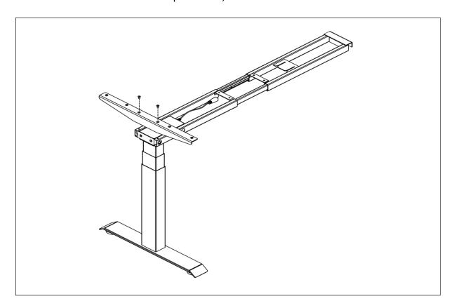
**Step 5**Connect the return frame to the single workstation and fixed with 2 hand bolts. Fix the centre brackets with 2pcs screws M6x10.
