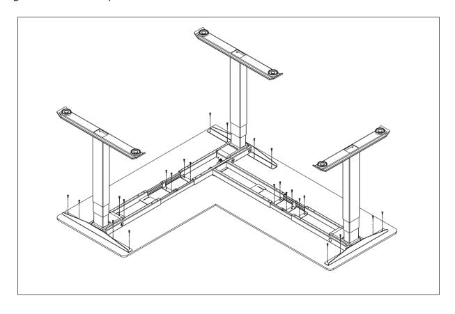
**Step 7**Mount the control box to the frame, fix the handset with 2pcs screws ST4x20.
