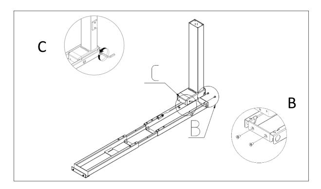
**Step 3**Install the table feet Screws 4 pcs M6x16,install the 4 leveling pads.
