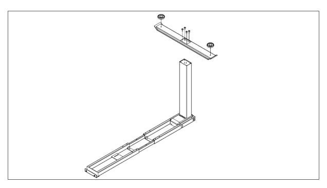
**Step 4**Install the side bracket with Screws 2 pcs M6x12,
