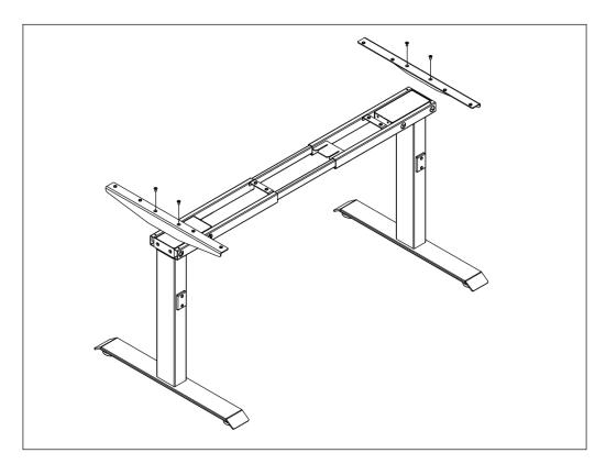
**Step 5**Mount the tabletop and fix it with 14 pcs screws ST4x20; Tighten the screws like D display to fix the top frame. Fix the centre bracket with 2 pcs screws M6x10
