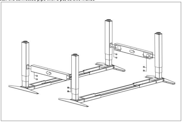
**Step 6**Fix the screen brackets with 8 pcs screws M6x10.
