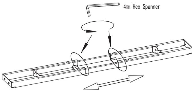
2 Attach the connecting beam connectors to the legs using 4 of M6\*10 screws, and attach the electric legs to the main beam using 8 of M6\*12 screws.
