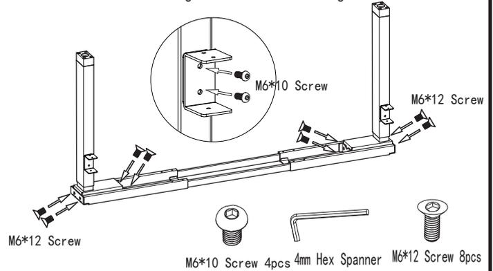
3 Attach the feet to the electric legs using 8 of M6\*40 screws.
