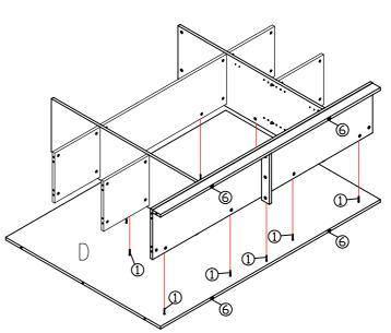
First insert the pin(part#1), then place the cam(part#2), and finally tighten/lock off after they have been put into
