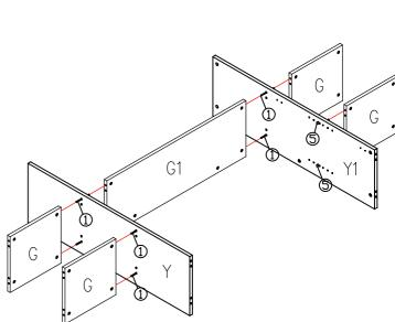
First insert the pin(part#1), then place the cam(part#2), and finally tighten/lock off after they have been put into the melamine.
